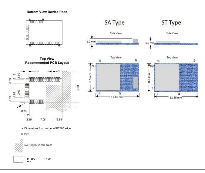
Note: Dimensions are in millimeters
