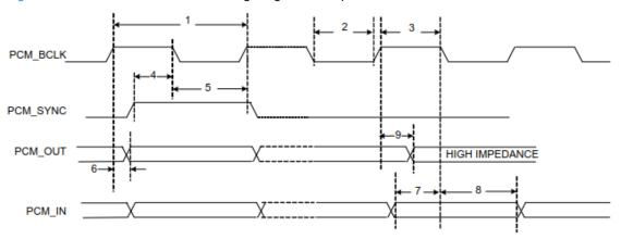
Figure 3: PCM timing diagram (Short-Frame Sync, Slave Mode)
