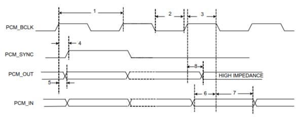
Figure 2: PCM timing diagram (Short-Frame Sync, Master Mode)
