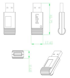
Figure 16: BT851 USB dongle, containing embedded BT850-SA
