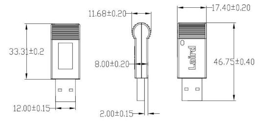
Figure 13: BT851 mechanical drawing
