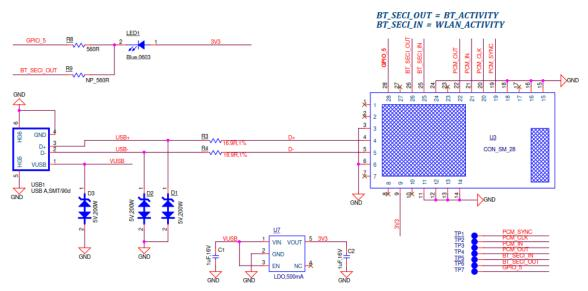
Figure 15: USB dongle design schematic
