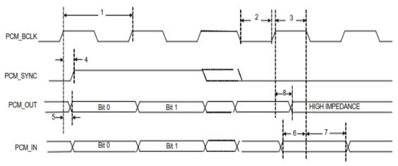
Figure 4: PCM timing diagram (Long-Frame Sync, Master Mode)
