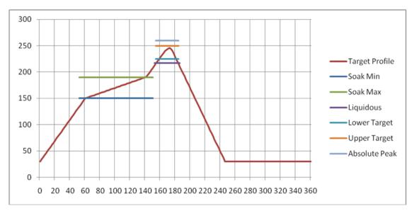
Figure 20: Recommended reflow temperature
