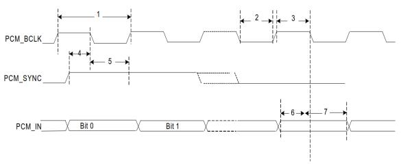
Figure 8: PCM burst mode timing (Receive Only, Long Frame Sync)
