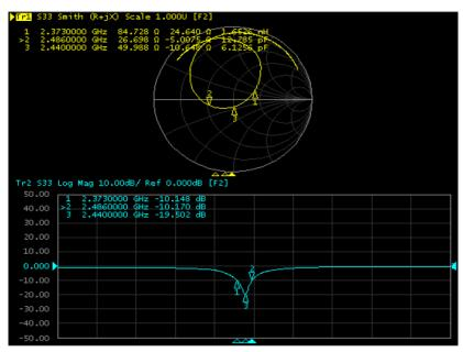
Figure 11: Antenna return loss
