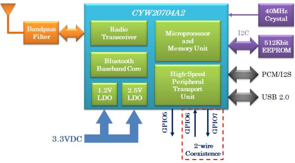
Figure 1: BT850 module block diagram
