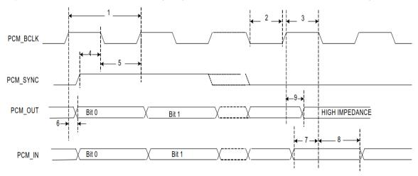
Figure 5: PCM timing diagram (Long-Frame Sync, Slave Mode)
