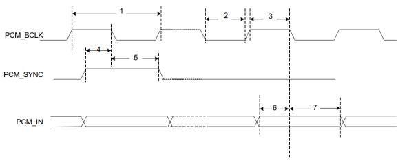
Figure 7: PCM burst mode timing (Receive Only, Short Frame Sync)
