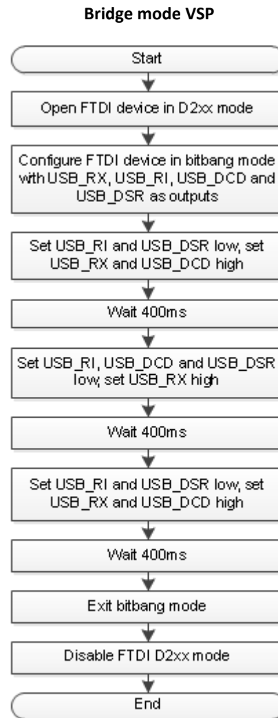
Figure 7: Flowchart for entering bridge mode VSP
