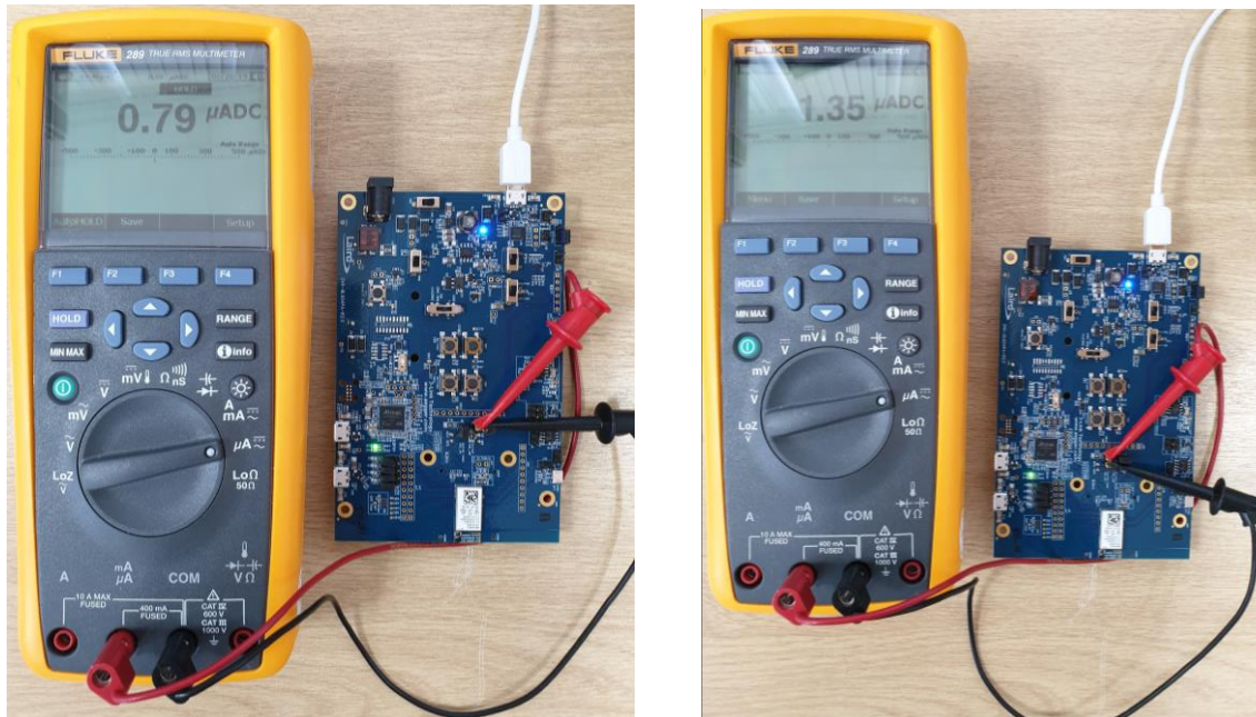
Figure 6: Deep Sleep mode current in Normal Voltage mode (VDD pin +VDD_HV pin) is 2.13uA total (=0.79uA + 1.35uA)
