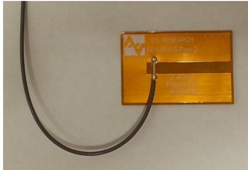
*Around the 'Cold' Side*
