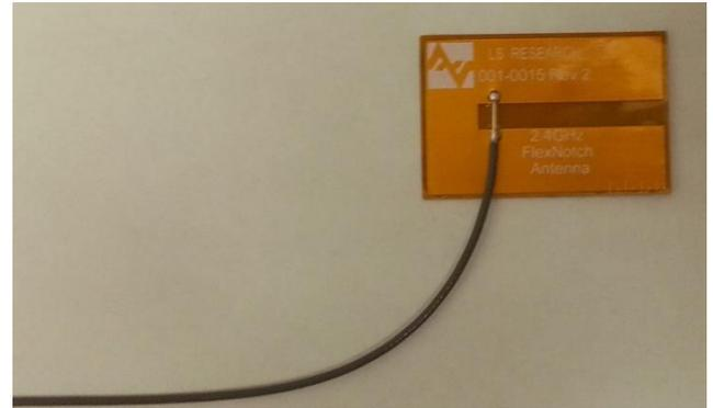
*Away from the Notch wall***Figure 15: Recommended cable routing**
