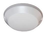
The Laird Connectivity S2451DBT is a dual-band six-element omnidirectional antenna for use in 802.11n MIMO applications. Three ports are designed to operate at 2.4 GHz and three ports are designed to operate at 5 GHz. Housed in a compact, low-profile radome, each of the six MIMO antenna elements is connected to the WLAN access point via a low loss, plenum-rated coax pigtail.
