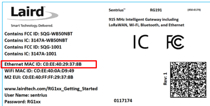
Figure 12: On a bottom label, M2 EUI corresponds to Serial number.
