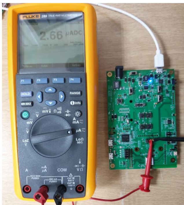
Figure 8: The current falls to about 2.6uA (2.54 uA to 2.86 uA is expected value) at 25°C temperature when placed in StandByDoze mode
