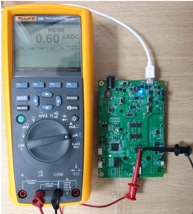
Figure 6: The current falls to about 0.6uA (600nA) at 25°C temperature when placed in deep sleep mode
