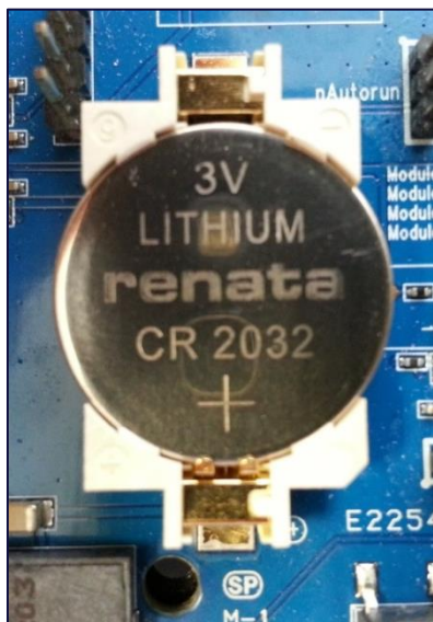
Figure 22: Inserting the coin cell (step 2)
