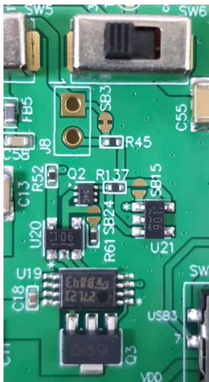
Figure 5: Schematic and PCB location of SB24
