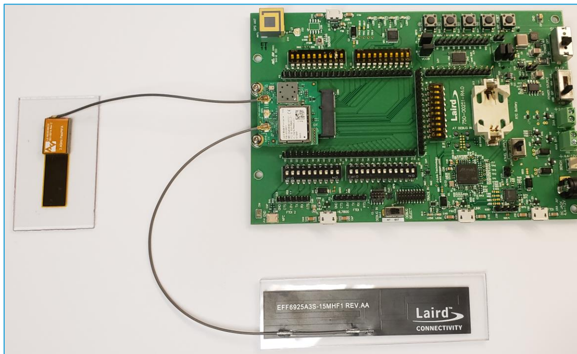
Figure 8: External antenna attachment for 453-00011 Pinnacle™ 100 modem
