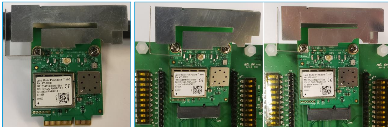
Figure 7: Attaching a 453-00010 Pinnacle™ 100 modem to a DVK
