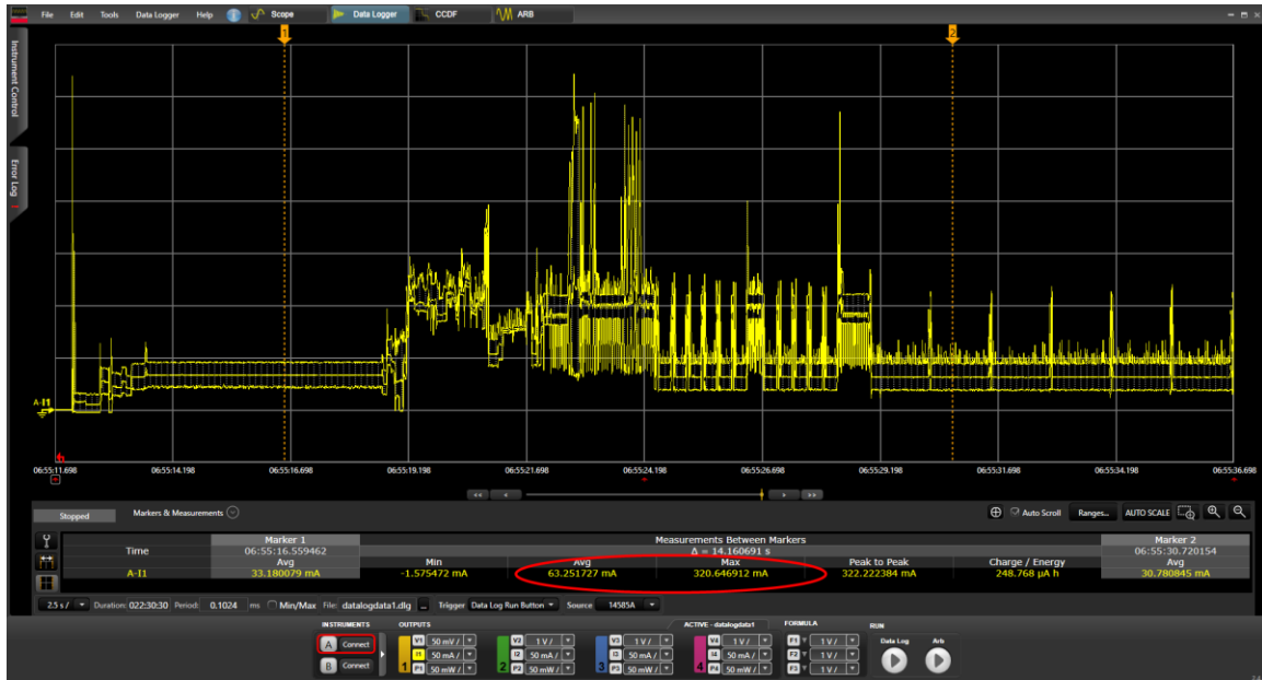
Figure 2: Pinnacle™ 100 Modem Current Profile for boot and establishing a connection
