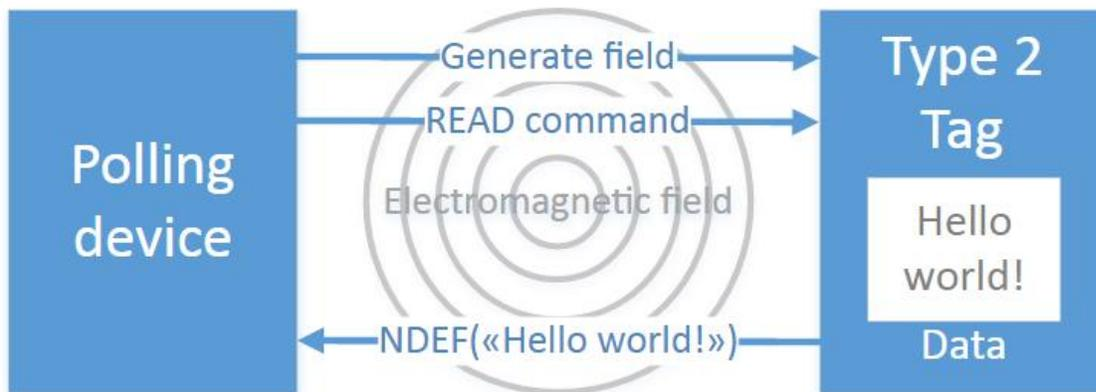
**Figure 9: Simplified overview of how NFC can be used**
