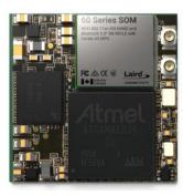
Laird's 60 Series SOM brings all of Laird's industry competence and capabilities into one solution. The SOM provides superior enterprise-class Wi-Fi connectivity with full support for 2x2 MU-MIMO 802.11ac WLAN, plus Bluetooth 4.2 dual-mode. This solution is equipped with a Cortex A5 applications processor, wireless and wired connectivity, enterprise-grade security, LCD support, and comprehensive Linux board support package (BSP).
