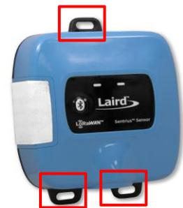
Figure 2: Front side of the Sentrius<sup>™</sup> RS1xx Sensor
