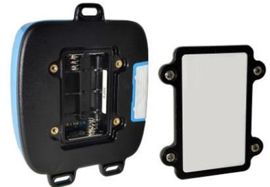
Figure 1: Back side of the Sentrius<sup>™</sup> RS1xx Sensor
