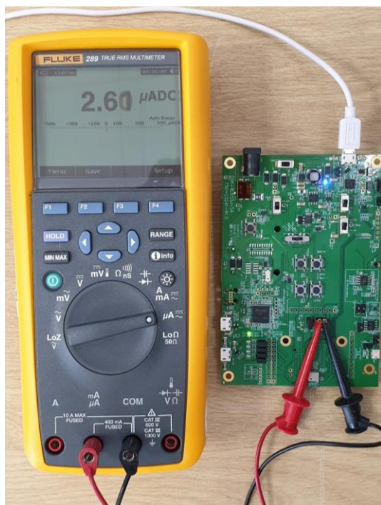
Figure 8: The current falls to about 2.6 \mu A (2.54 \mu A to 2.86 \mu A is expected value) at 25°C temperature when placed in StandByDoze mode
