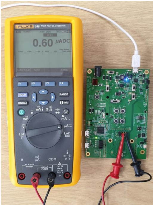
Figure 6: The current falls to about 0.6 \mu A (600nA) at 25°C temperature when placed in deep sleep mode
