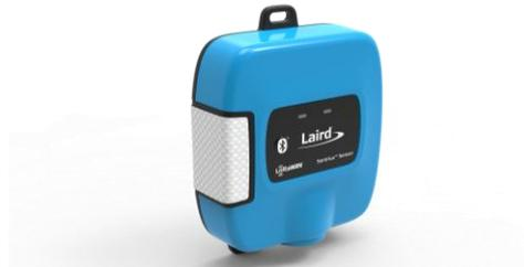
The Sentrius™ RS1xx Series LoRa/BLE sensor features integrated antennas, temperature and humidity sensors in rugged enclosures.
