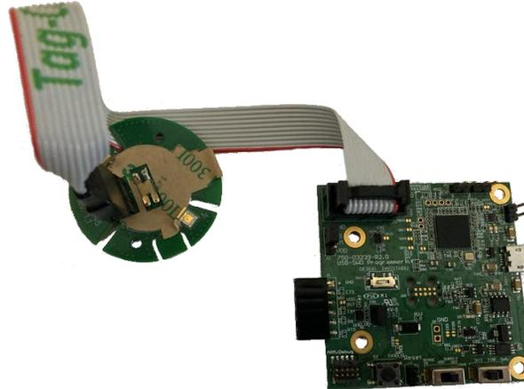
Figure 2: BT510 connected to USB-SWD Programmer Board with test mode enabled
