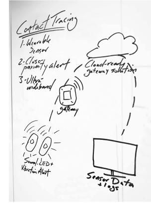
What was missing was how to capture that alert data and route it to the cloud. This missing piece would enable the key component of a next-gen social distance monitoring system: up-to-date cloud logging of non-compliances (events where two users cross the safe distance threshold and trigger an alert). This is critical if a user gets sick - the cloud log of interactions can help compile a list of who else may have been exposed, enabling them to quarantine and reduce spread of the disease.
