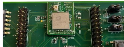
Figure 1: 455-00030 Sterling-EWB Development Kit w/ Chip Antenna
