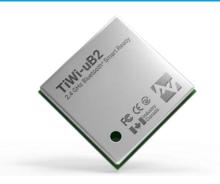
The TiWi-uB2 Bluetooth® Smart Ready module is a high performance 2.4 GHz Bluetooth 2.1+EDR and Bluetooth Low Energy radio in a cost effective, precertified footprint. This module fully supports the dual mode Bluetooth and Bluetooth LE operation, and the output power can support class 1.5. This ultrasmall SiP module provides UART interface/audio PCM interface for Bluetooth through the HCI transport layer.
