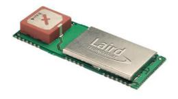
The Embedded Bluetooth® AT Module is designed for applications that demand arobust and reliable Bluetooth connection. This product is designed with solder connections for mounting directly onto a main PCB. The integrated high-performance, multilayer ceramic antenna is highly resistant to de-tuning, allowing great flexibility in positioning.
