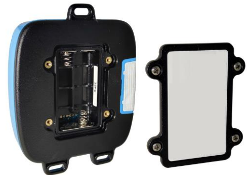
Figure 2: Back side of the Sentrius RS1xx sensor
