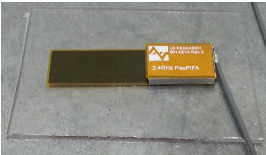
Figure 26: FlexPIFA mounted on metal Surface with 1.5 mm thick polycarbonate spacer
