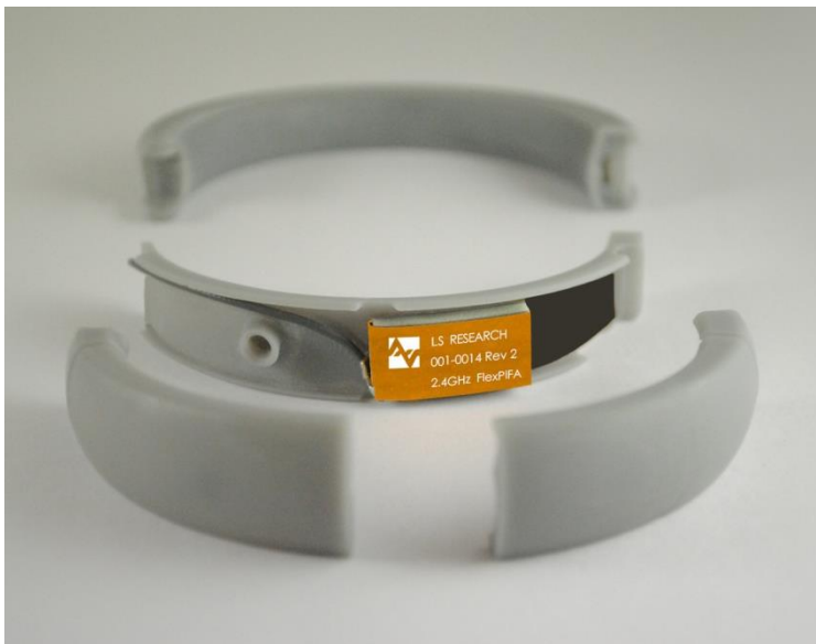
Figure 28: FlexPIFA integrated into bracelet
