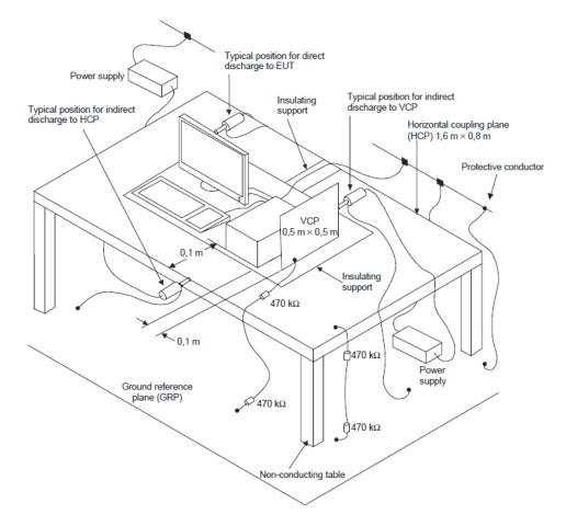
The test setup shall consist of a non-conductive table, (0.8  $\pm$  0.08) m high, standing on the ground reference plane.
