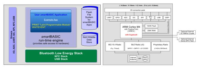
Figure 1: Bluetooth smartBASIC module block diagram
