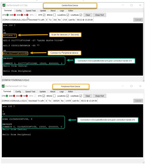
Note: For an explanation of the connection response see section 3.4.1.1 of the AT Interface User Guide. The number following "CONNECT" is the connection handle.
