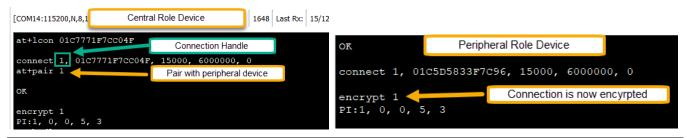
Note: For explanation of response to pairing see section 3.4.3.30 of the AT Interface User Guide.
