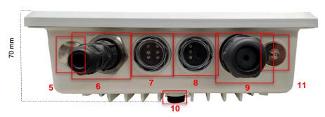
Figure 60: Side panel of the IP67 Rated Sentrius™ RG1xx LTE Gateway (Current Generation)
