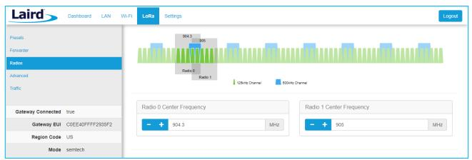
Figure 36: Channel assignments
