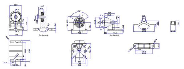
Figure 74: Pole mount dimensions
