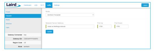
Figure 34: Semtech packet forwarder configuration
