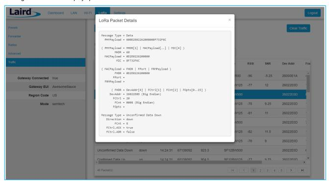
Figure 45: LoRa packet details
