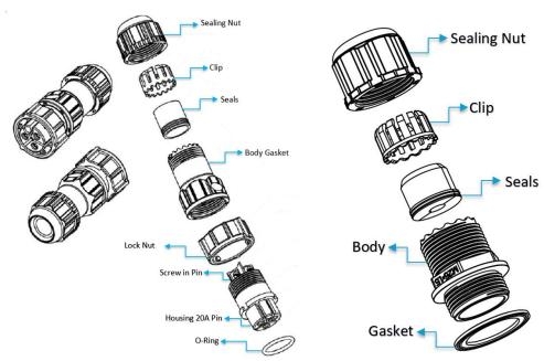
Figure 64: Power cable (left) and Ethernet (right) assembly components
