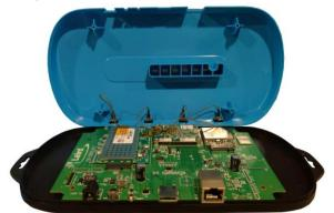
Figure 5: Opened Gateway (indoor (non-IP67) gateway shown)
