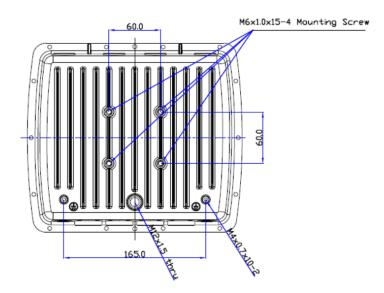
Figure 72: Enclosure placement dimensions (mm)
