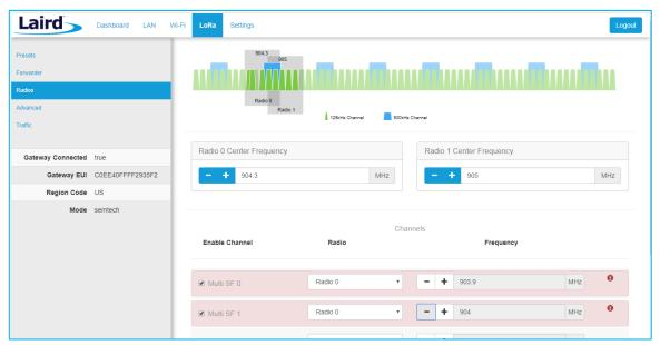
Figure 38: Overlapping channels
