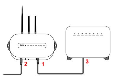
Figure 3: Connecting the gateway
