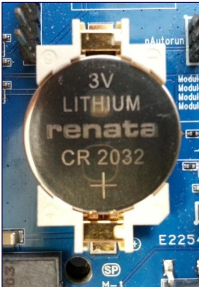
Figure 22: Inserting the coin cell (step 2)
