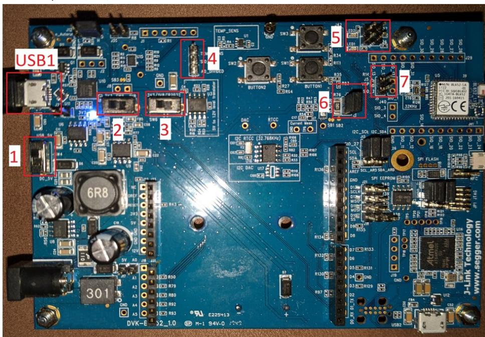
Figure 1: Switch and jumper positions for the BL652
