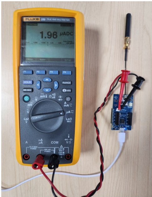
Figure 6: RM1261 LoRa PCB Module Sleep current at 25°C temperature with AT firmware
