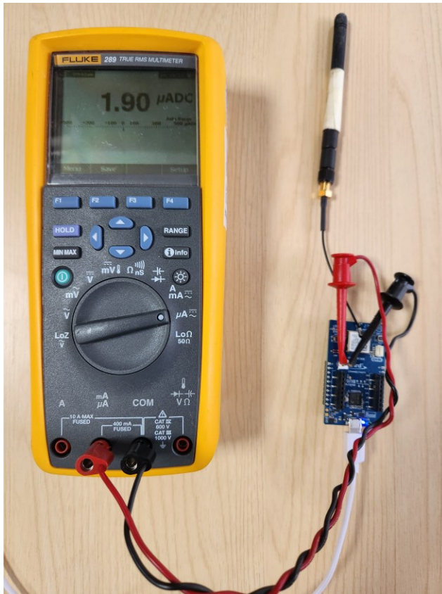
Figure 7: RM1262 PCB Module Sleep current at 25°C temperature with AT firmware
