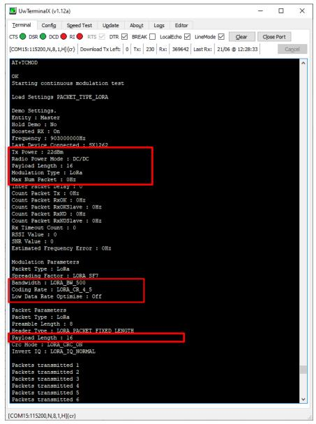
Figure 5: Configured for TX Test LoRa 500kHz Modulated signal (RF duty cycle is not 100%) and Start Test
