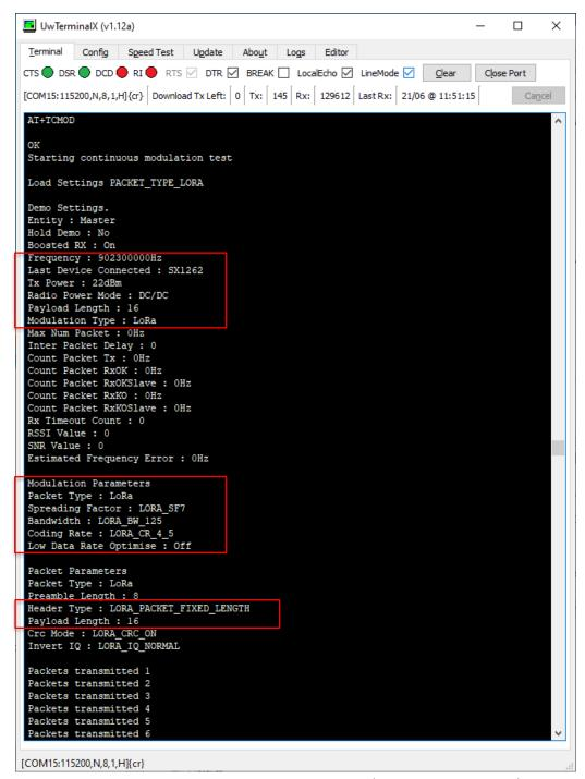
Figure 4: Configured for TX Test LoRa 125kHz Modulated signal (RF duty cycle is not 100%) and Start Test
