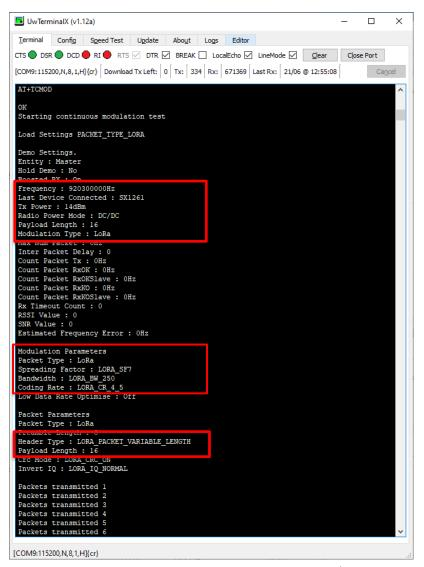
Figure 6: Configured for TX Test LoRa 250kHz Modulated signal (RF duty cycle is not 100%) and Start Test
