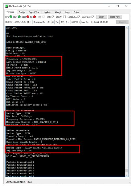
Figure 7: Configured for TX Test FSK 50kbps Modulated signal (RF duty cycle is not 100%) and Start Test
