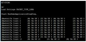
Both units exchange data until test is stopped on either unit or packet count value reached.
