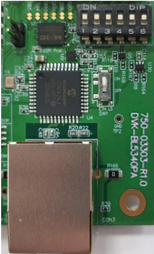
Figure 18: SPI device Ethernet chip (U4), level shifters (U30, Q5, U9), closed DIP switch (S5) schematic and PCB
