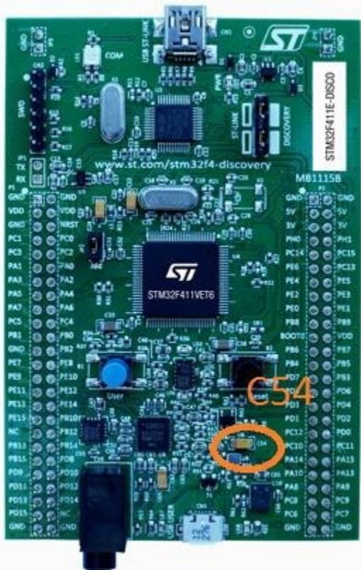
Figure 3: Remove C54 From Discovery Board
