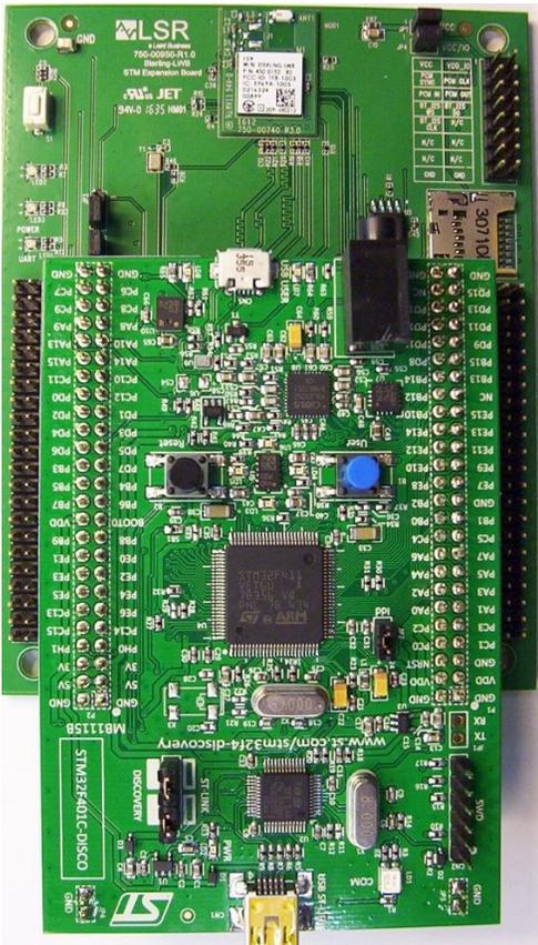
*Figure 4: Discovery Board Connected to Expansion Board*
