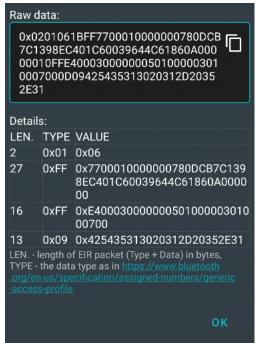
This advert payload is composed of three different Data Types (0x01,0xFF, 0x09) that all contain one or more bytes of value. For more information on different Bluetooth GAP Data Types, you can refer on  $\underline{\text{Generic Access Profile}}$ .
