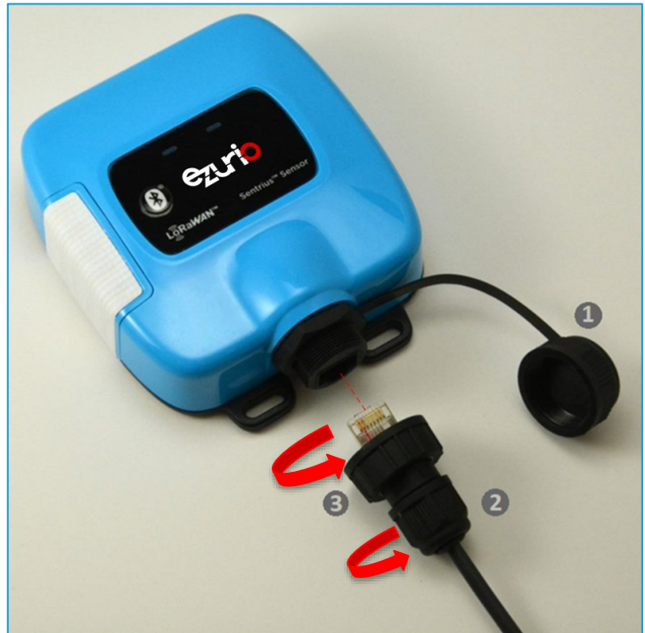
Figure 3: Installing the external Open/Closed sensor
