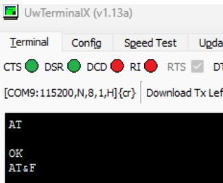
Figure 4: UwTerminalX: AT and AT&F command usage
