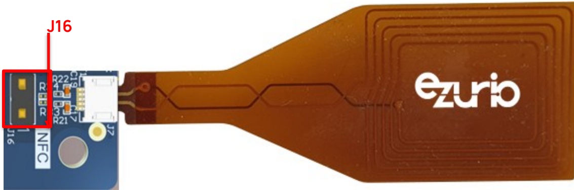
Figure 8: NFC antenna RF matching circuit, NFC antenna connector schematic and NFC plugged in to connector J7
