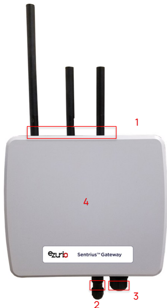
Figure 59: Top of the IP67 Rated Sentrius™ RG1xx Gateway
