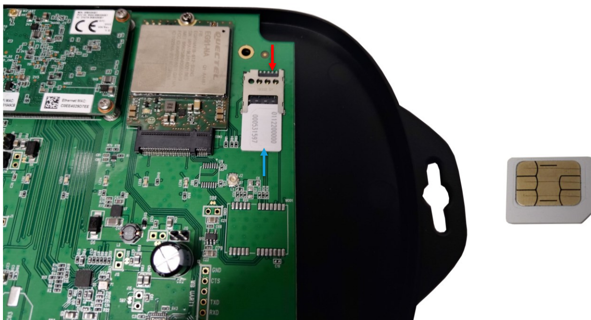
Figure 7: SIM Install (Right: Picture of SIM card contact side)
