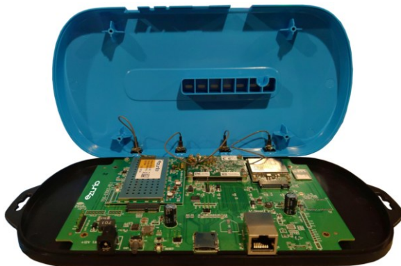
Figure 5: Opened Gateway (indoor (non-IP67) gateway shown)
