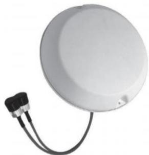
The CMD69273P, using patent-pending technology, is an indoor broadband low PIM 2-port MIMO omnidirectional ceiling mount antenna. It is designed to provide pattern coverage optimized for indoor requirements at 698-960 MHz and 1710-2700 MHz frequency bands. The individual antenna elements are designed with linear H/V-polarization components oriented to radiate a pattern that has been specifically shaped to deliver optimal performance from a ceiling mount location.
