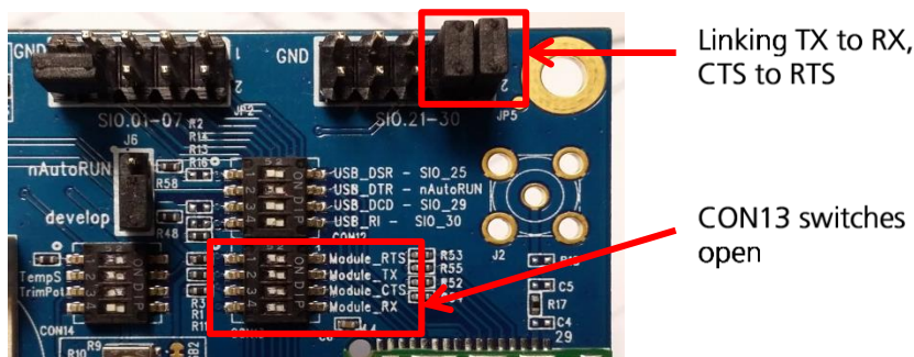
Figure 4: Devkit setup for Cable Replacement Mode with Loopback
