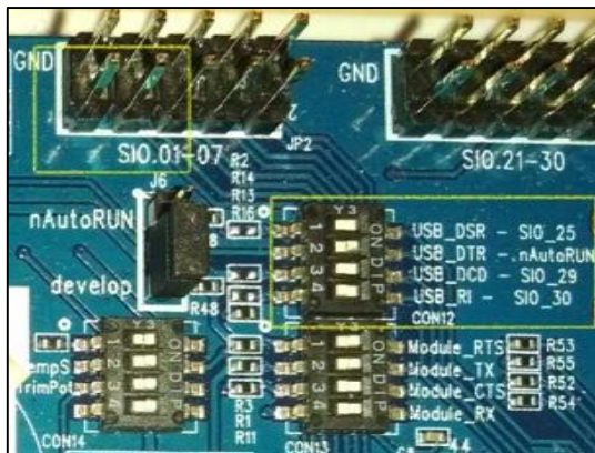
Figure 1: SIO7 tied to VCC using a jumper and CONN12 Switch 2 ON
