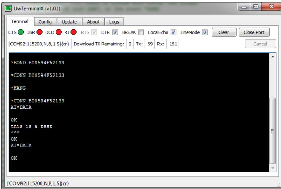
Figure 7: Switching between Bridged and Command modes
