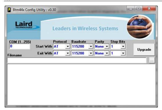
Change the COM port as per the setting in the PC for the dev kit, specify the protocol and COM port parameters for 'Start With' and 'Exit With', select the filename in the appropriate text box (which may be automatically selected if there is only one .dfu file in the same folder as the utility) and then click **Upgrade**.
