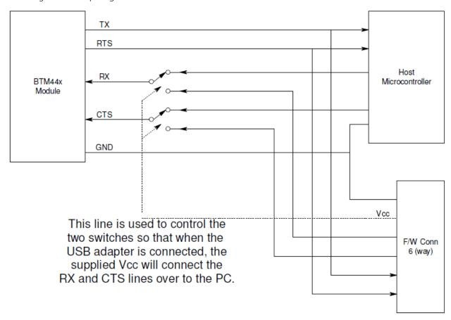
In this arrangement the extra cost to the bill of materials consists of components that implement the multiplexing of the RX and CTS lines. This multiplexing can be via a header/jumper arrangement or it can be logic gates driven by the Vcc line of the 6 way USB F/W Conn that allows the USB to Serial adapter to gain control of the BT module.
