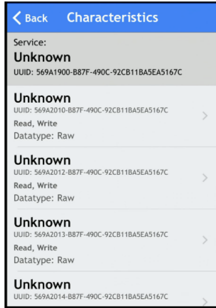
Figure 9: Characteristics within service (BLExpri)
