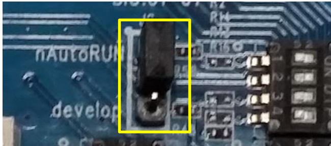
Figure 6: Jumper position for Autorun mode
