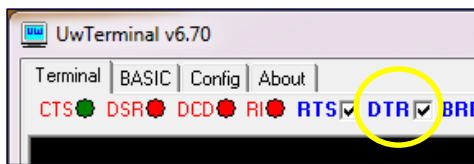
Figure 5: Asserting DTR line in UwTerminal
