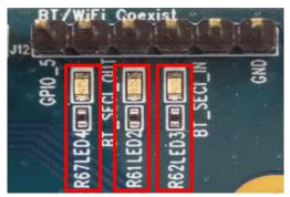
Figure 4: LED2, LED3, LED4
