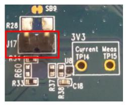
Figure 9: Current measurement circuit
