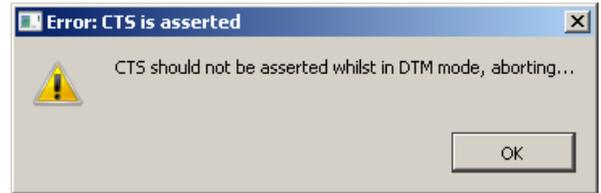
Figure 4: Module not detected as being in DTM mode
