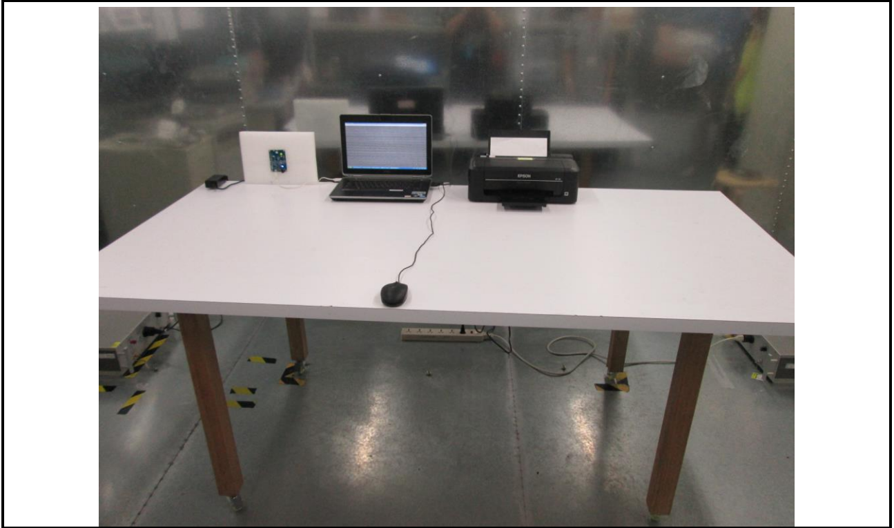
Conducted Emission Test (Model: BT830-SA with antenna 1)
