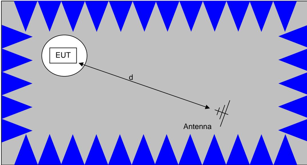
The anechoic materials on the walls and ceiling ensure compliance with the normalized site attenuation requirements of CISPR 16 / CISPR 22 / ANSI C63.4 for an alternate test site at the measurement distances used.
