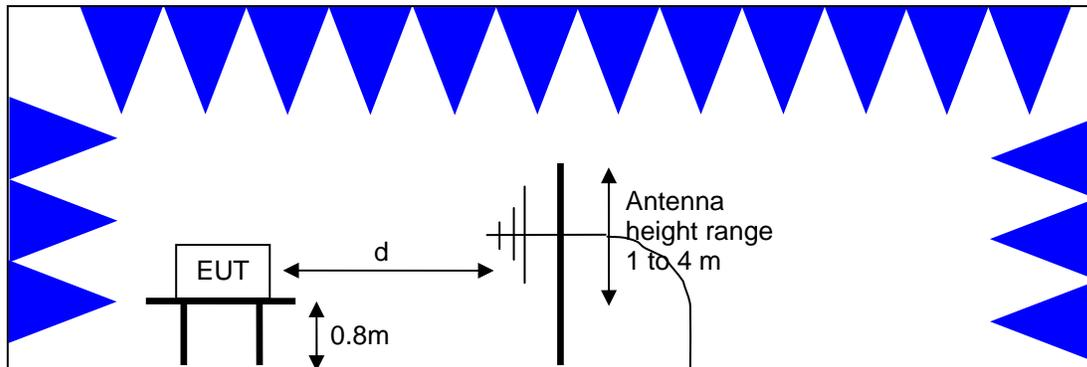
Test Configuration for Radiated Field Strength Measurements
