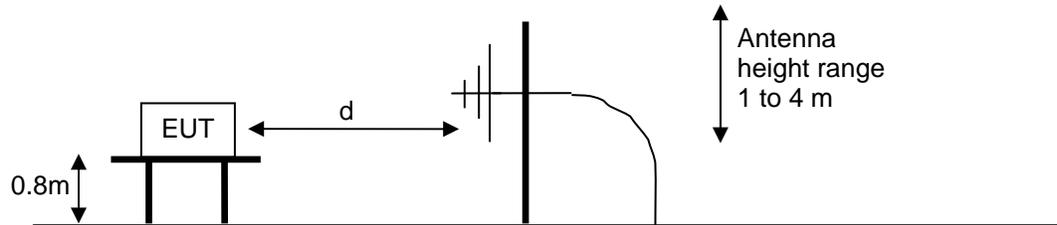
Test Configuration for Radiated Field Strength Measurements
