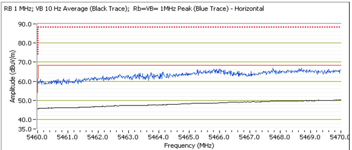
Note 1: For emissions in restricted bands, the limit of 15.209 was used. For all other emissions, the average limit was set to -27dBm/MHz (-68dBuV/m).
