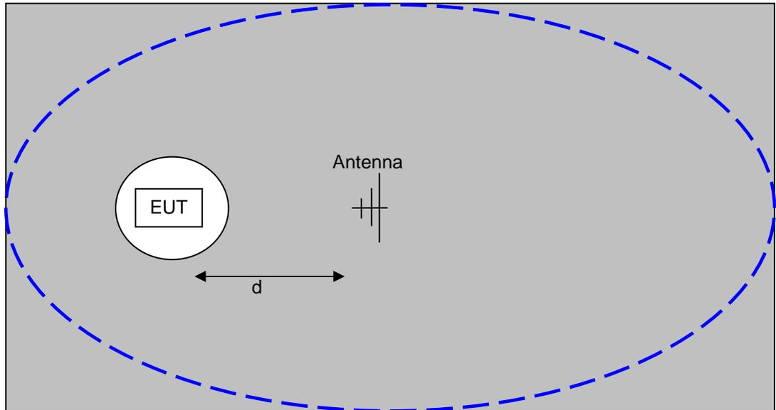
The ground plane extends beyond the ellipse defined in CISPR 16 / CISPR 22 / ANSI C63.4 and is large enough to accommodate test distances (d) of 3m and 10m. Refer to the test data tables for the actual measurement distance.
