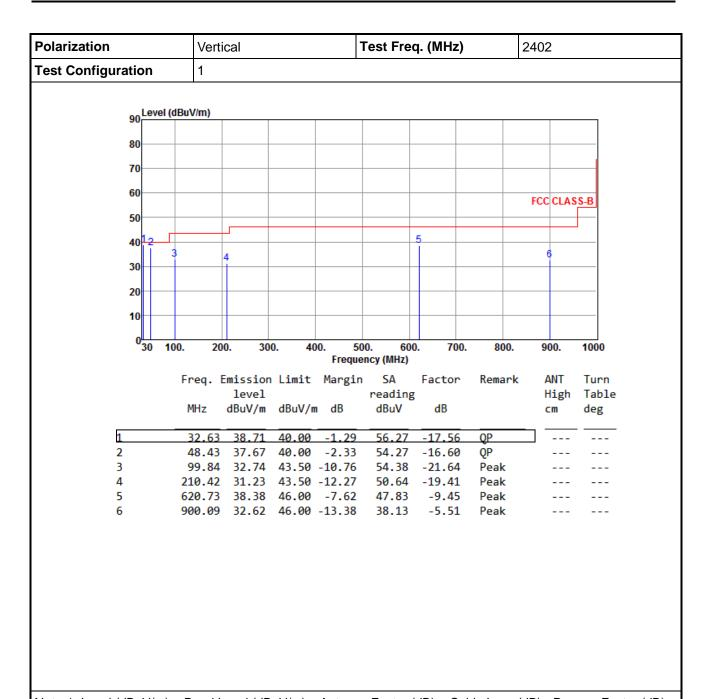
Note 1: Level (dBuV/m) = Read Level (dBuV/m) + Antenna Factor (dB) + Cable Loss (dB) - Preamp Factor (dB). 2: Over Limit (dBuV/m) = Limit Line (dBuV/m) - Level (dBuV/m).
