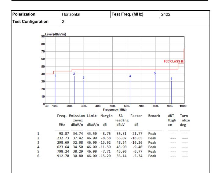
Note 1: Level (dBuV/m) = Read Level (dBuV/m) + Antenna Factor (dB) + Cable Loss (dB) - Preamp Factor (dB). 2: Over Limit (dBuV/m) = Limit Line (dBuV/m) - Level (dBuV/m).
