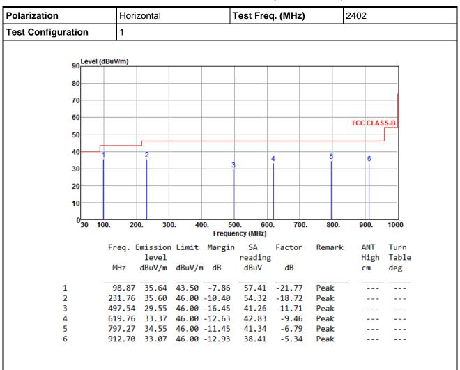
Note 1: Level (dBuV/m) = Read Level (dBuV/m) + Antenna Factor (dB) + Cable Loss (dB) - Preamp Factor (dB).
