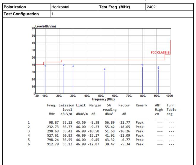
Note 1: Level (dBuV/m) = Read Level (dBuV/m) + Antenna Factor (dB) + Cable Loss (dB) - Preamp Factor (dB).
