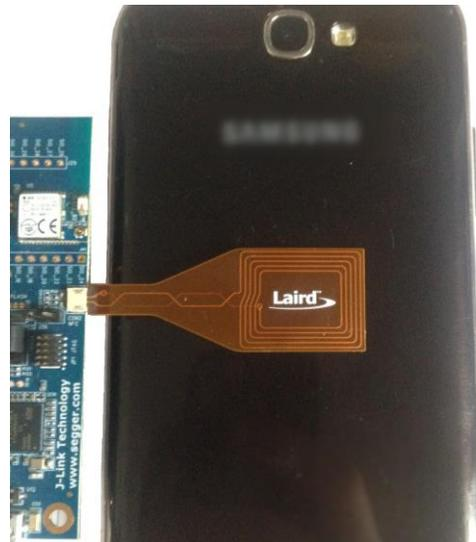
Figure 12: BL652 NFC antenna held flush against android device
